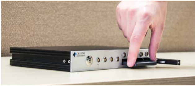
The Spider-NAS features eight dedicated high-speed data buses and a removable 250 GB serial ATA (SATA) Solid State Disk (SSD).
