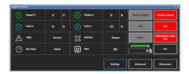
The amplifier status is recorded in Run Logs, which appears in EDM software, report, and EDM Cloud for in-test view, post-test view, and remote view.
