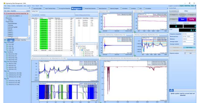
Figure 3. Hammer Impact Measurement of the disc brake rotor
