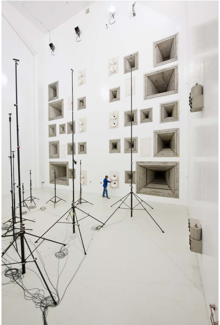
Figure 1.1 - RATF (Reverberant Acoustic Test Facility) at NASA Plum Brook (courtesy of NASA)
