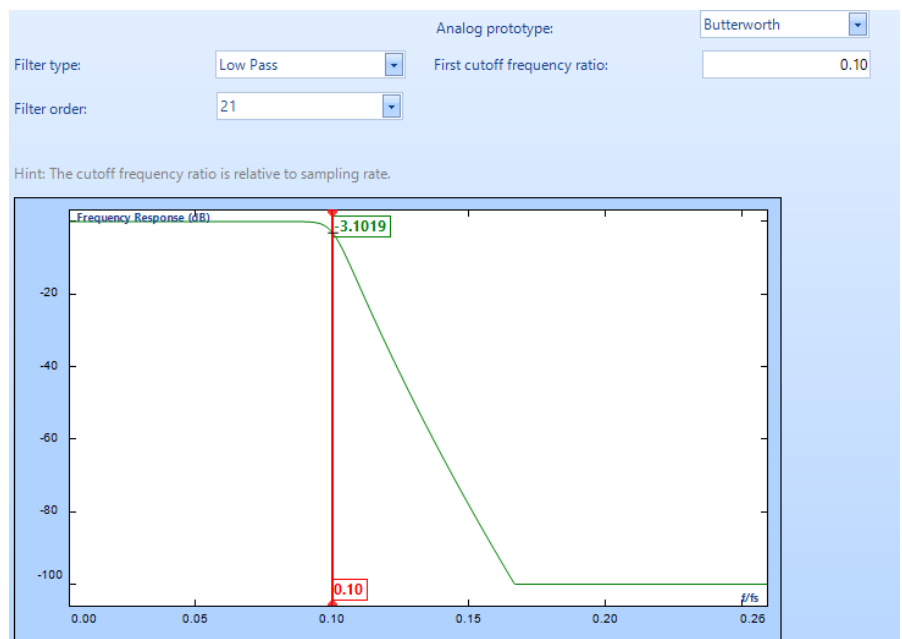
Figure 60. Butterworth low pass filter
