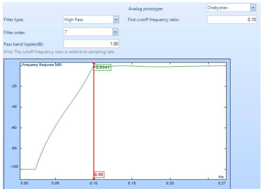
Figure 62. Chebyshev type I high pass filter
