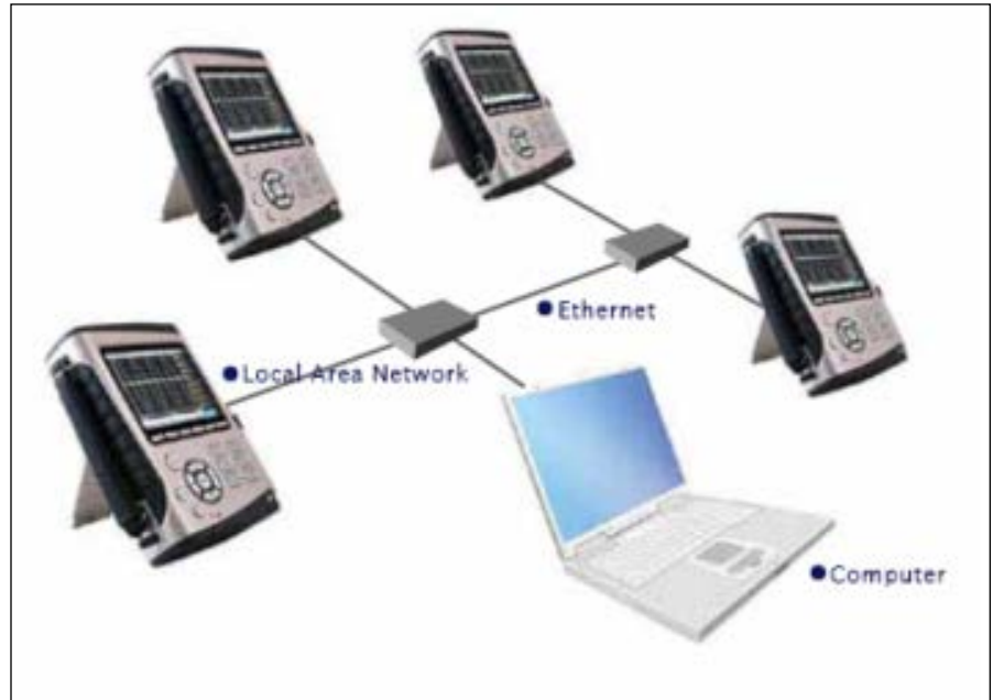
Figure 46. Remote operation for multiple CoCo DSA units with automated testing
