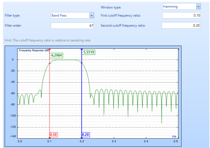
Figure 53. Hamming window method
