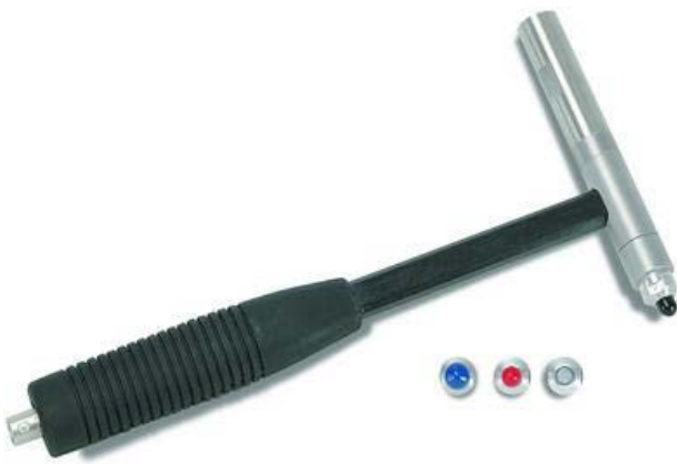
Figure 7. Impact hammer instrumented with a force sensor with different hardness tips.
