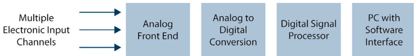
Figure 20. Signal analyzer architecture
