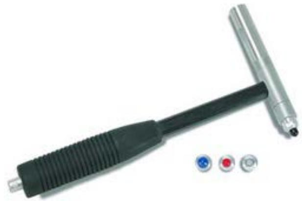
Figure 17. Impact hammer instrumented with a force sensor to measure the excitation force and different hardness tips
