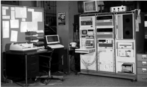
Figure 3. HP5451 dynamic analysis system.
