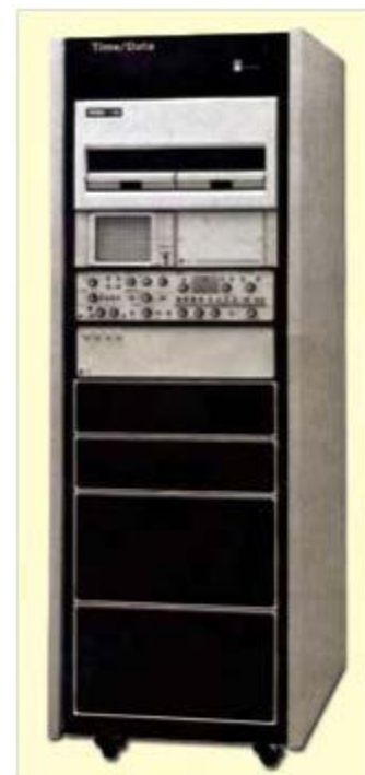
Figure 5. GenRad Time/Data TDV 20 vibration control system.
