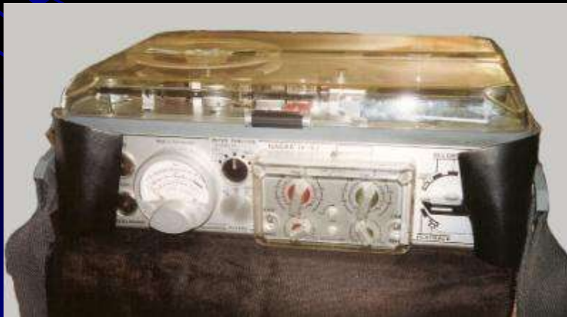
Nagra two channel magnetic tape recorder used in early predictive maintenance programs (in carrying case).
