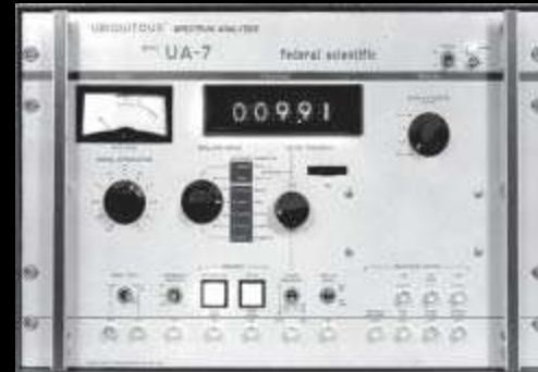
60s: The first commercial RTA from Federal Scientific was the UA-7 Ubiquitous® Spectrum Analyzer.
