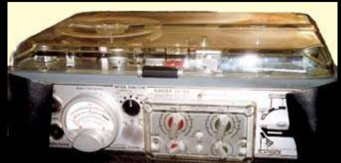
The portable, two channel direct (AM) tape recorder manufactured by Kudelski in Switzerland,
