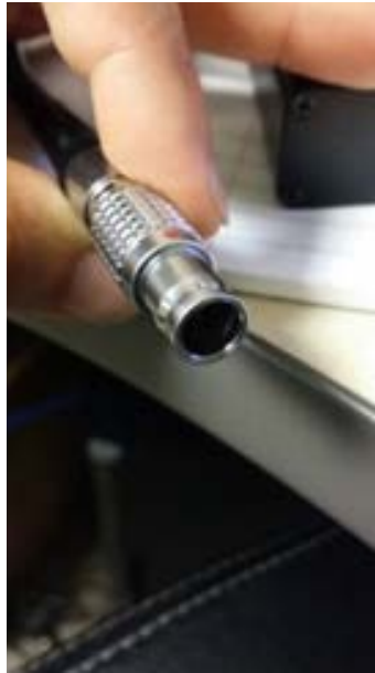
Figure 1.3 1 of 8 included Input Channel Adaptors, a breakout box to interface gage wires
