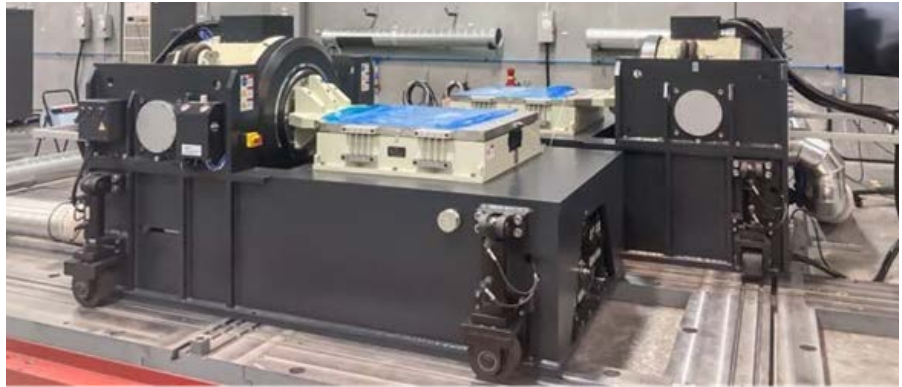
Figure 1.2 Rail system allows shakers to be rearranged in different configurations
