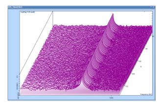
The reference axis of the 3D signals can be customized with time or RPM.
