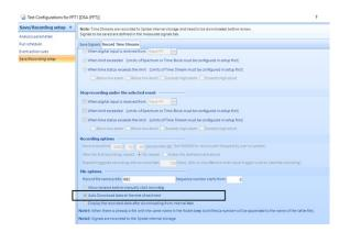
As soon as the test ends, recordings from the internal flash can now be auto downloaded without having to manually select and download the data.
