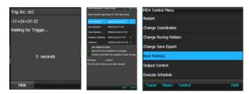
Modal Data Acquisition (MDA) is a dedicated user interface for entering impact testing coordinates during testing. Geometric coordinates are stored in the file header, allowing easy importing into supported modal mode
