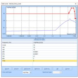
Limits can now be set on individual Octaves and the Magnitude of FRF signals. Limits are implemented on DSP making the limits capable of running even in the black box mode.
