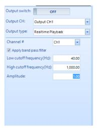
Any channel can be selected to be played back at any of the input. A band pass filter can also be applied to the output signal while playing back.
