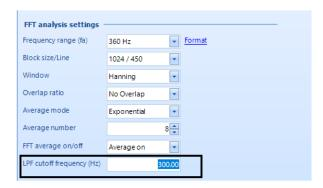
User can now define a Low Pass Filter (LPF) for filtering out the
