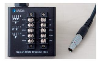
3 –wire configurations help to compensate the wire resistances associated with the strain gages and also compensate for the changes in the wire resistances due to temperature or other factors during the course of the test.
