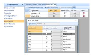
lected response signals would exceed the given limits if the input acceleration specification were followed, the input acceleration is reduced.
