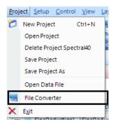
Post Analyzer can be used with signal files recorded on a variety of instruments using a variety of acquisition devices. File Converter is a convenient platform to convert a range of file types to ATFX file type (common file type used for EDM and PA).
