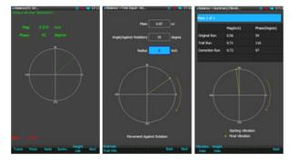
Rotor balancing allows correcting the unbalance without having to dismantle the machine. It is possible to balance rotors of any size with either 1 or 2 plane balancing. Using the 'multiple channel' option, parallel measurements on 2 sensors are possible, resulting in a faster, safer and more accurate procedure. The user interface allows stopping and starting balancing as wanted and to perform again any single operation without running the whole procedure.
