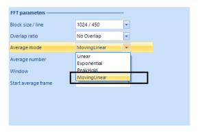
Moving Linear Average also called rolling linear average is now introduced in PA. With this option, linear averages are computed for the selected frame count and the test does not pause when the average number is reached. Instead, the test continues computing the linear average of the most recent frame number similar to the Exponential averaging mode.
