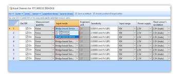
The sensitivity of strain gage based sensors are typically ratiometric and depends on the excitation voltage.
