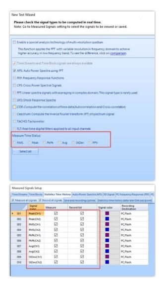
These signals are available as time history signals, which allows these signals to be recorded to the PC in real time. Thus, these signals can be viewed for the entire duration of the test during any point of the test or after the test is complete.
