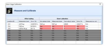
EDM 9.0 introduces a user-friendly window to detect any obvious errors which can denote an incorrect connection or a bad sensor.
