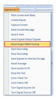
Users can set the channels requiring offset correction. Some sensors reading static pressure, torque, or displacement data should not be nulled. This feature allows the user to select sensors that need to be offset corrected.
