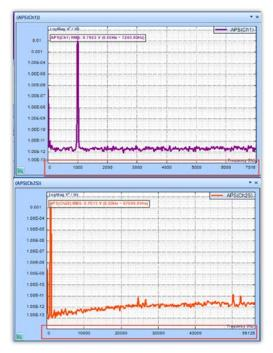
The variable sampling rate is useful with strain, temperature, and displacement sensors where frequency domain signals are not of prime importance.
