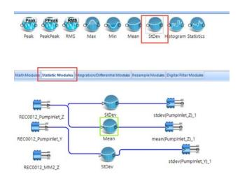
Users can add standard deviation to any number of channels. In addition, a channel can be customized to calculate the standard deviation in addition to mean or any other property or module.
