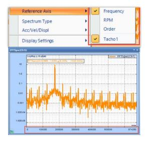
A choice of tachometers is also available to enable the selection of either tachometer as the reference.
