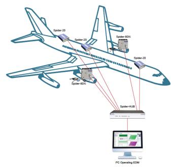
The Spider-20 series of products are ultra-portable and can be mounted at even remote locations. The Spider-80X and Spider-80Xi on the other hand are powerful front-ends that can chain together to obtain simultaneous data acquisition for up to 1024 channels.
