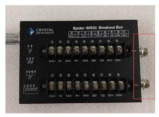
The provided break-box is convenient for custom connecting strain gages or any of the supported sensor types.
