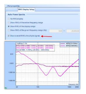
The total energy in signals acquired through sensors specialized for different frequency ranges can be acquired and the overall energy can be estimated.
