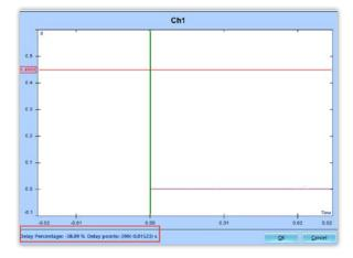
The cursors can now be used to accurately adjust the pre-trigger.
