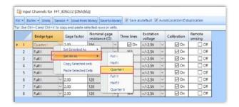
It is now possible to simultaneously set the bridge type, gage factor or any of the strain gage related parameters. This feature will greatly simplify the strain gage configuration for high channel count systems.
