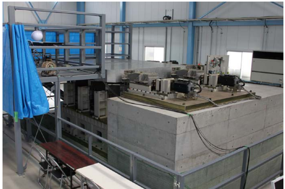
Figure 1.2 Nissoku Engineering Co., Ltd Three-Axis Servo Shaker System
