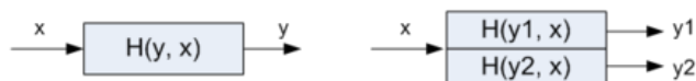
Figure 1: Left - a UUT with one response; Right - a UUT with two responses
