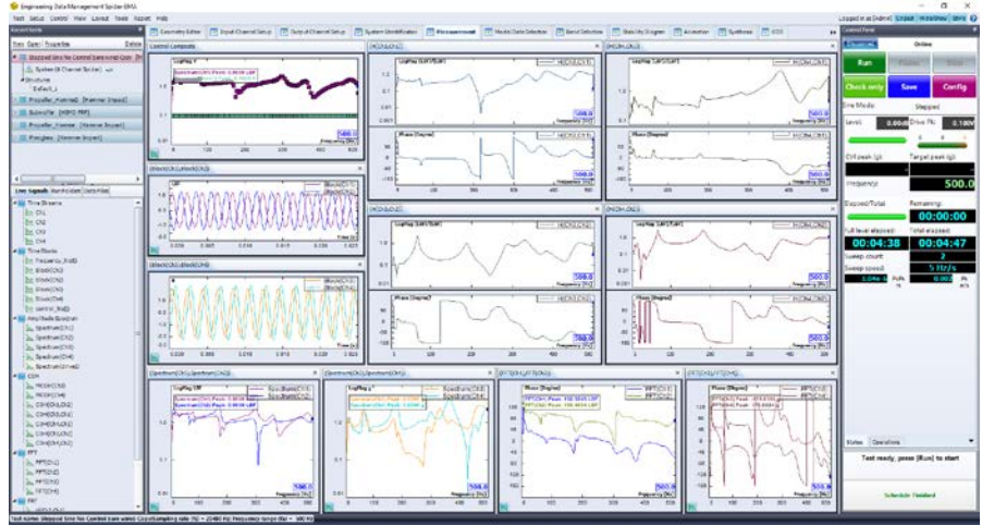
Figure 1.13 - MIMO Sine Excitation for GVT modal measurements on aircraft
