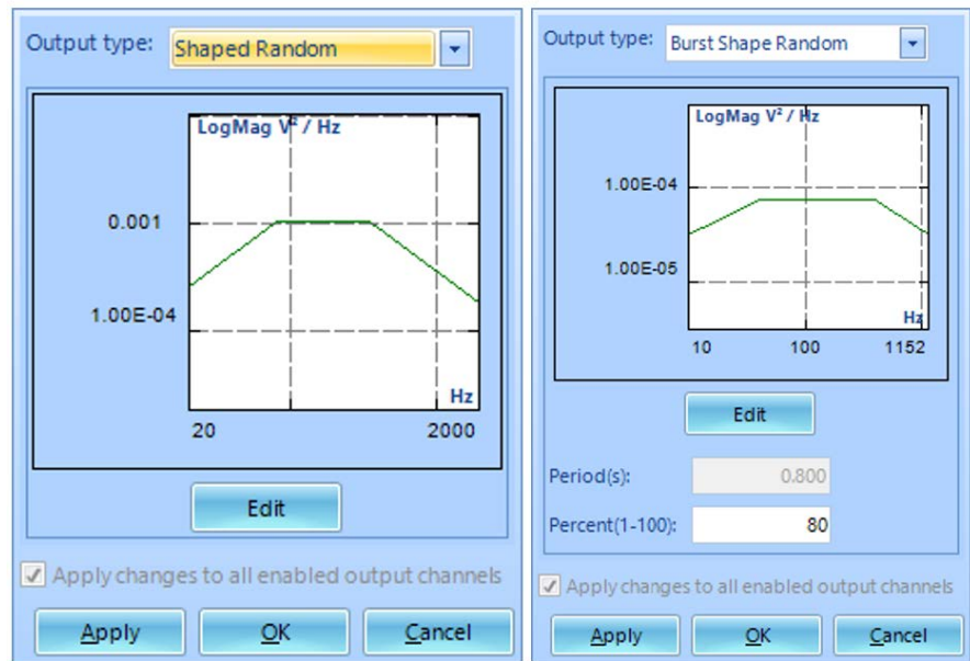
Figure 1.11 - Shaped Random & Burst Shaped Random Excitation for plugging in a PSD drive profile
