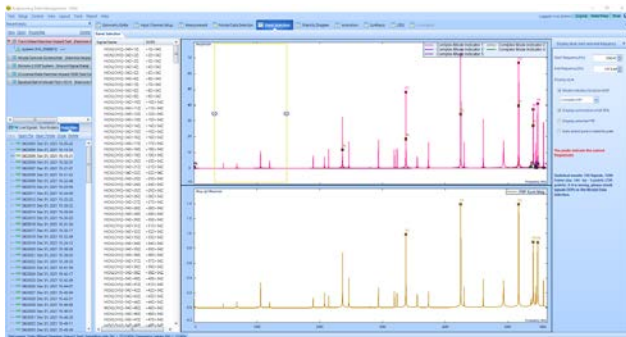
Figure 5. Mode Indicator Functions to locate and identify the modes in the desired frequency range
