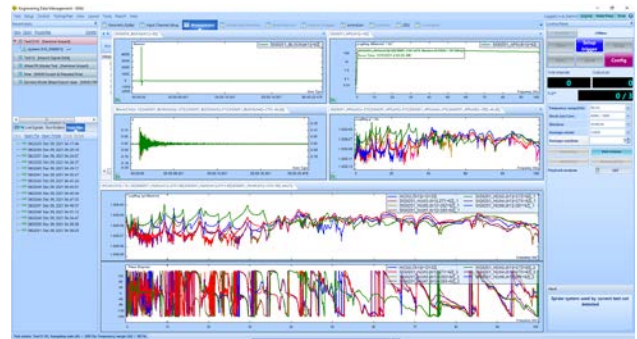
Figure 3. Hammer Impact Measurement of the Processing Equipment
