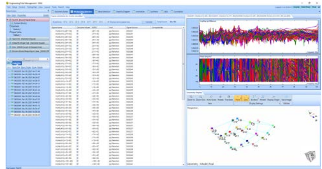
Figure 4. Modal Data Selection tab showing the overlapped FRFs
