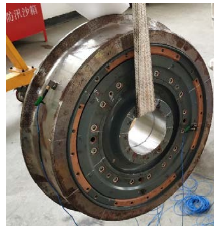
Figure 1. Modal hammer testing of the train wheel
