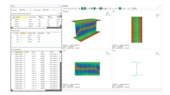
The mode shape animation can be set to different speed and amplitude using the animation control icons. In addition, the different geometry display features can be used to provide a good visual effect of the animation.
