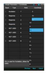
The above screenshot shows the mapping between input channels and the geometric coordinates. Two coordinate types are available: XYZ or RTP. Both coordinate types can be assigned positive or negative directions.
