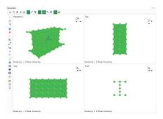
On the top and bottom plate, the measurement is carried out along the Z direction. While on the middle plate, the measurement is carried out along the +Y direction. There are total of 63 points on this I-Beam geometry model.
