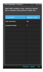
The above page allows the user to set the roving pattern. In theory, the user can set the geometric coordinates manually without automatic roving. But for most tests with hundreds of geometric points, manually entering the coordinates would be too time-consuming. The CoCo MDA provides methods to automate this process.
