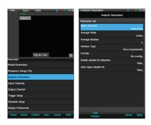
Select the appropriate block size, average mode and average number. Note that the selection of window type must be either Uniform or Force-Exponential for impact hammer testing.
