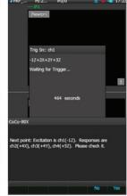
Using the impact hammer, hit point 7 with an appropriate amount of force. Observe the signal qualities. You can carefully examine the signal quality by selecting each trace.
