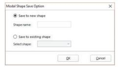
The coming mode shape can be saved to a new shape data file, or saved to an existing shape data file. In general the modal analysis process is done through multiple bands, and the mode data can be saved to an existing shape data file. This will result in one shape data file containing all the mode data over the complete frequency range.
