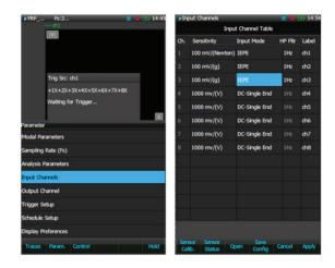
Channel 1 is connected to the impact hammer so therefore the sensitivity should be set to mV/Newton. Channel 2 and 3 are connected to accelerometers with IEPE power enabled.
