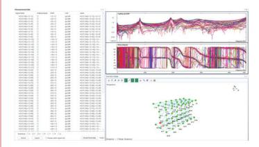
The FRF signals from each measurement can be displayed one by one, or all together. The current corresponding response point will be highlighted on the geometry model as a red dot.
