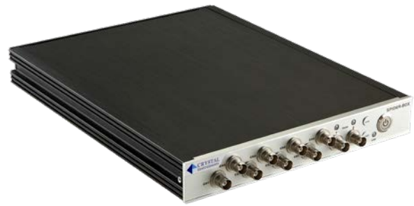
Figure 7. Spider-80X module accepts eight analog signals and two tachometer signals through front panel BNC connectors; it provides a power switch and status LEDs (power, run/stop, flash memory capacity, LAN communication).
