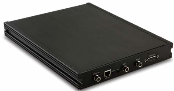
Figure 8. Rear panel provides a 100Base-T female RJ45 Ethernet connection, a LIMO five-pin Spider-NAS port, an RS-485 serial port, a DB25 Digital I/O connector and a 15 VDC ( \pm 10\% , 10 watt) power input connector.
