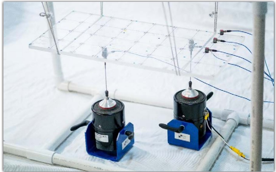
Figure 1.1 Modal Shaker Testing of the plexiglass plate
