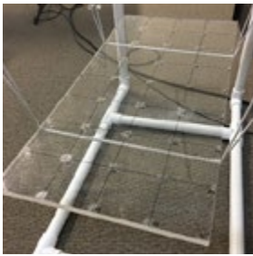
Figure a. free-free suspension of plexiglass board
