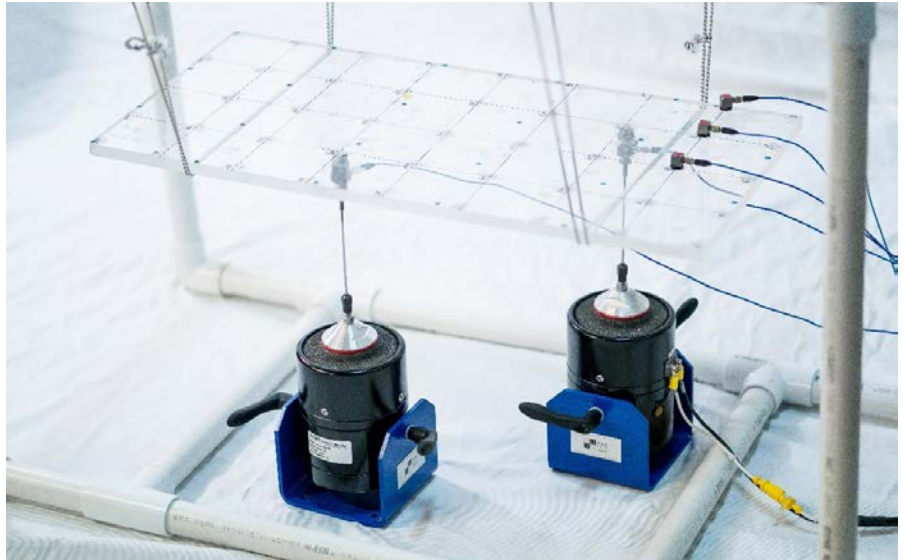
Figure 3.1 Plexiglass board free-free suspension on a test bench
