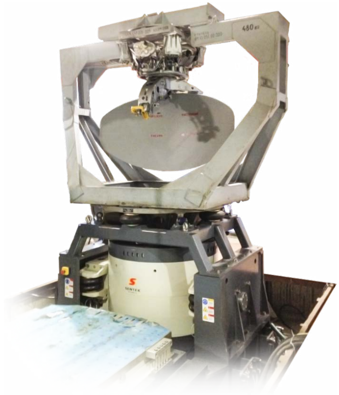
Figure 7.1 Vertical configuration for a sine vibration test
