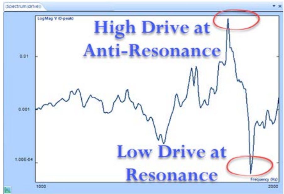
Figure 5.1 Dynamic range in a controller
