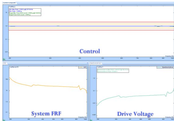
Figure 4. Single axis sine vibration control test in EDM VCS Sine
