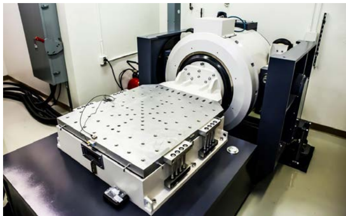
Figure 22. Horizontal configuration for a sine vibration test
