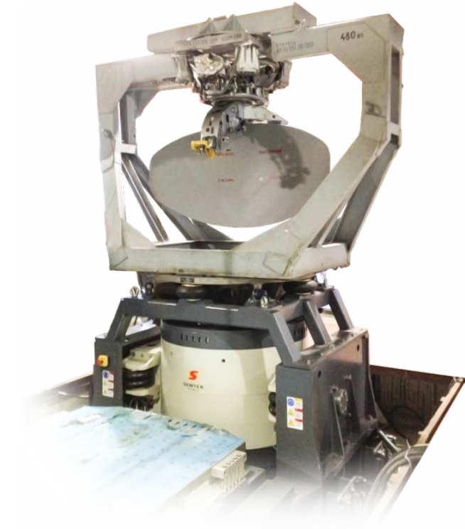
Figure 21. Vertical configuration for a sine vibration test
