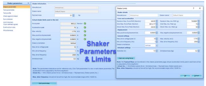
Figure 23. Setup of shaker parameters and shaker limits
