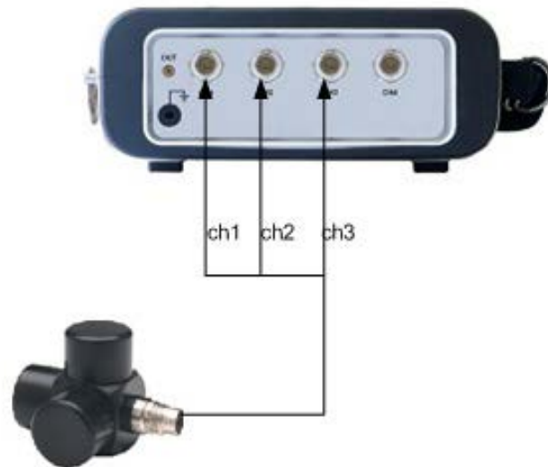
Figure 2.5 Connecting Tri-axis Accelerometer
