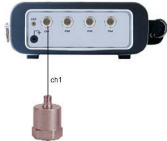
Figure 2.4 Connecting Channel 1 to Accelerometer
