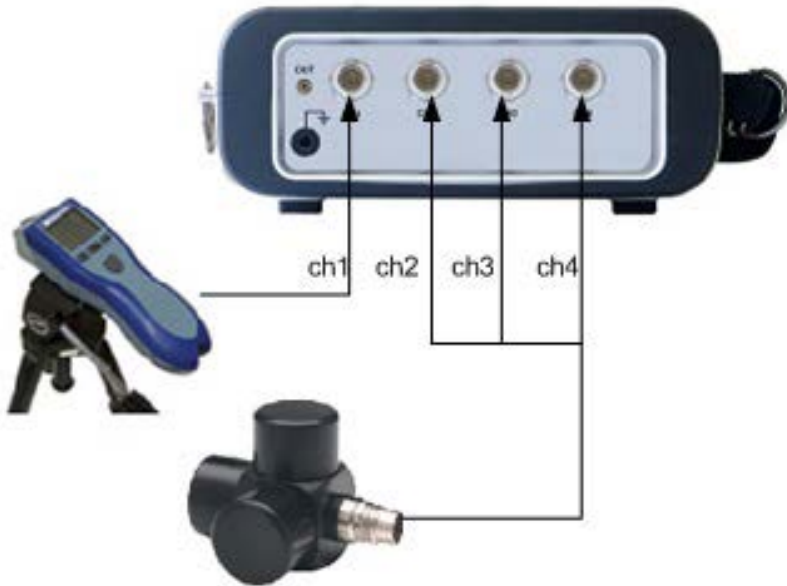
Figure 2.7 Connecting Tachometer and Tri-axis Accelerometer
