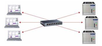
**Case 7:** Multiple PCs connected to a multiple Spider system, each spider system has multiple chassis
